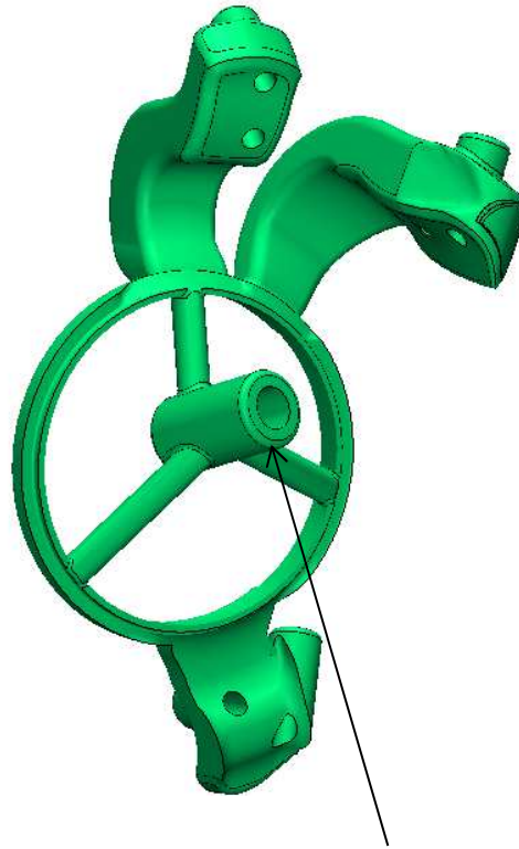
1 hole for Ø6mm drill
